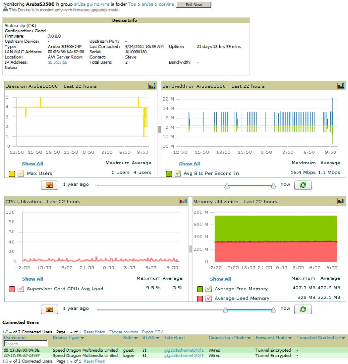
Figure 96 APs/Devices > Monitor Page for a Mobility Access Switch
